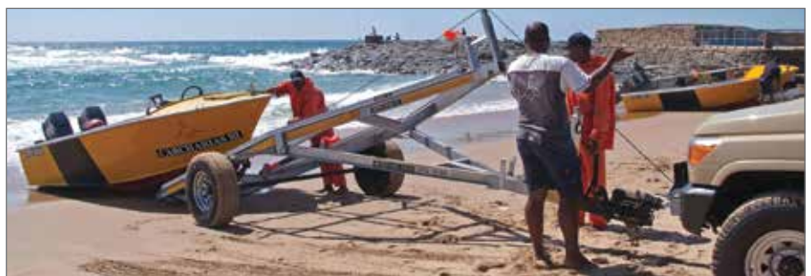
Photo 3: Use of break-back trailer and 4x4 with front-mounted winch and tow hook (Photo courtesy Natal Sharks Board)
