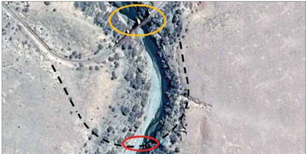
Figure 4: The permanent bridge position is marked yellow, the temporary bridge site red, and the approximate position of the deviation by a dashed line (Google Earth, annotated Johannes Haarhoff)
