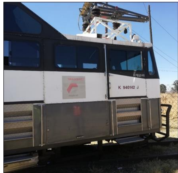
Figure 3: Luxrailer inspection Trolley
