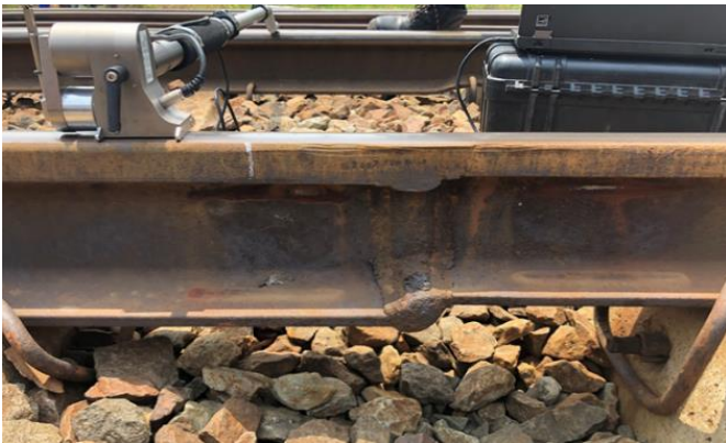
Figure 4: Thermite junction rail profile measurements
