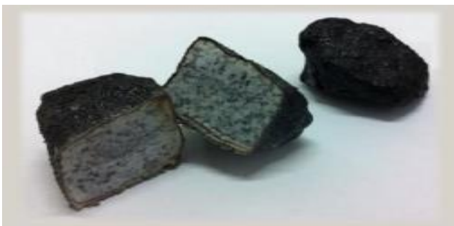
Figure 2. Ballast coated in rubber particles i.e. Neoballast (Valentí, et al., 2016)
